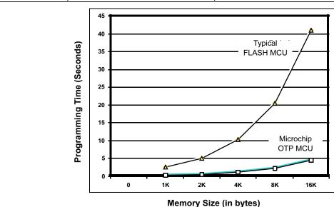
**Note 1:** The programming times shown here only include the total programming time for all memory. Typically, a programmer will have quite a bit of overhead over this "theoretical minimum" programming time.
