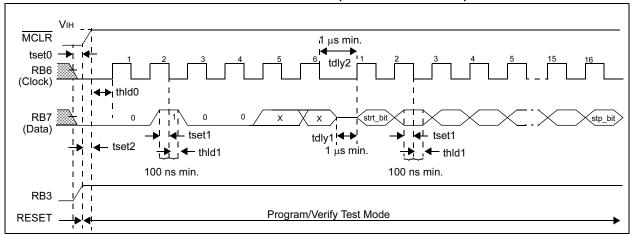
FIGURE 6-5: READ DATA COMMAND MCLR = VDD (PROGRAM/VERIFY)
