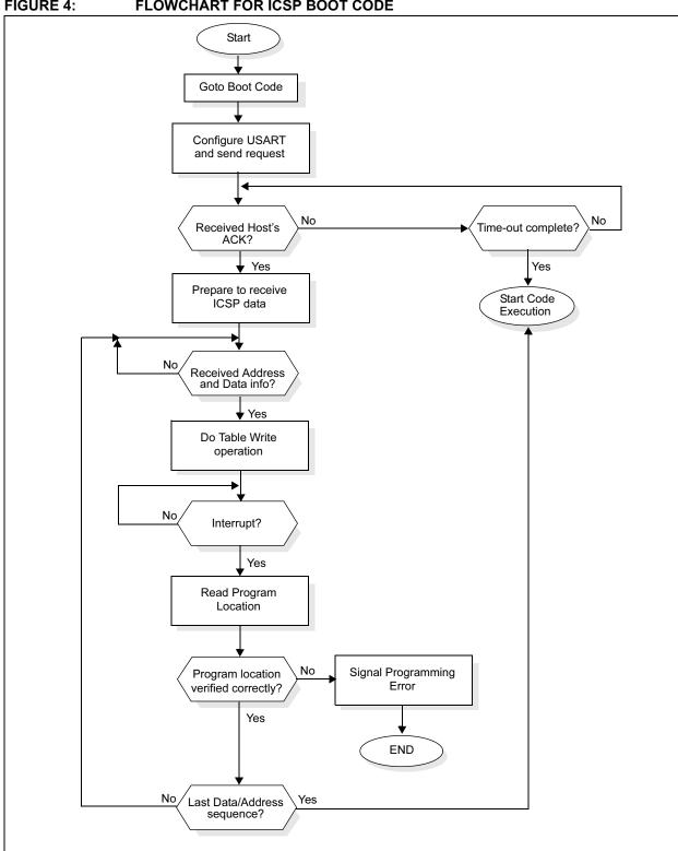
FIGURE 4: FLOWCHART FOR ICSP BOOT CODE
