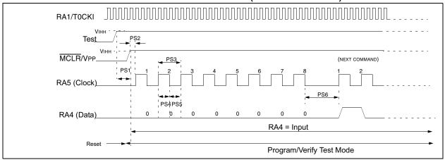
FIGURE 7-2: INCREMENT ADDRESS COMMAND (PROGRAM/VERIFY)
