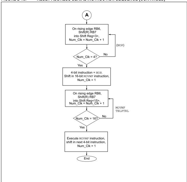
FIGURE 2-16: RESET ADDRESS SERIAL INSTRUCTION SEQUENCE (CONTINUED)
