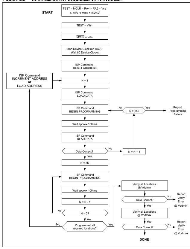
FIGURE 4-8: RECOMMENDED PROGRAMMING FLOWCHART
