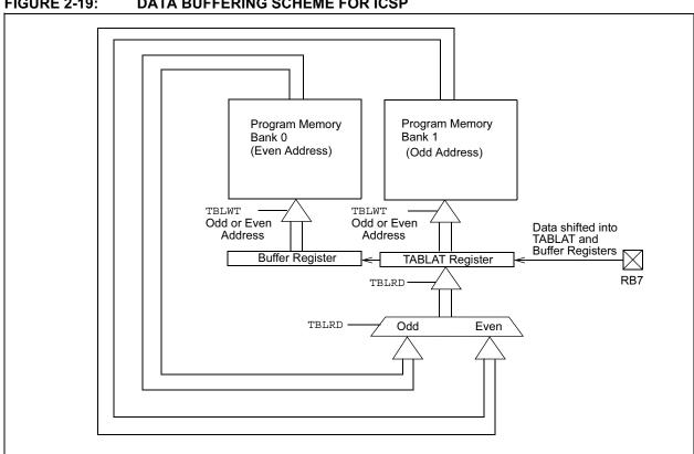
**FIGURE 2-19:** DATA BUFFERING SCHEME FOR ICSP
