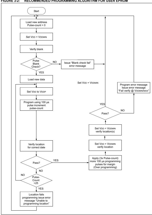
FIGURE 3-2: RECOMMENDED PROGRAMMING ALGORITHM FOR USER EPROM
