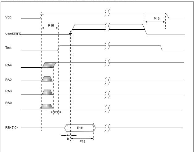
FIGURE 6-4: POWER-UP/DOWN SEQUENCE FOR PROGRAMMING
